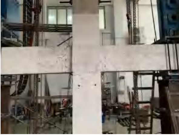
(c) 裂缝宽度增大，柱端产生裂缝
